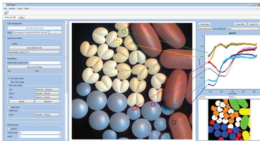
RGB true color rendering with imec snapscan hyperspectral imaging software with spectra plotted out and classification of a sample of various pharmaceutical pills
